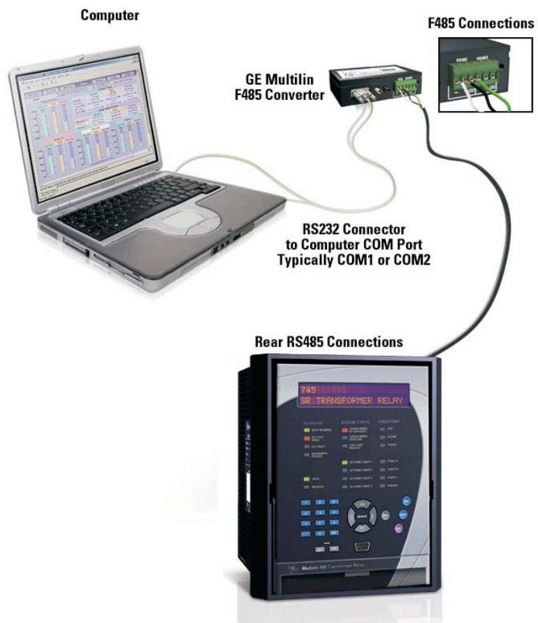
FIGURE 4-3: Communications using rear RS485 port
