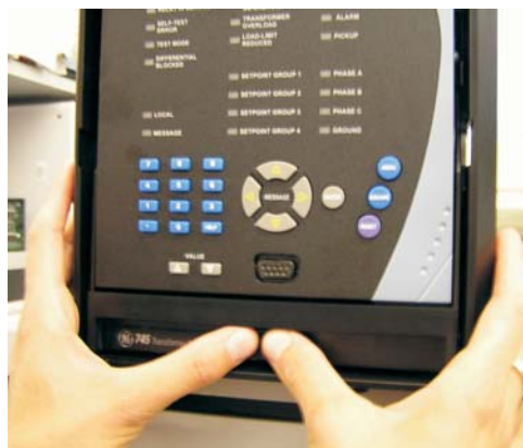
FIGURE 3-5: Press latch to disengage handle
