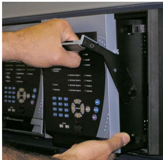
FIGURE 3-7: Slide unit out of case
