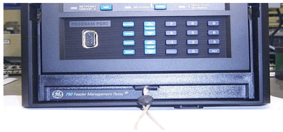
FIGURE 3-8: Drawout unit seal
