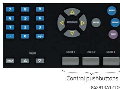
Figure 5-10: CONTROL PUSHBUTTONS (ENHANCED FACEPLATE)
