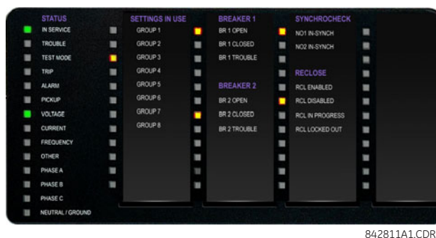
Figure 4-18: TYPICAL LED INDICATOR PANEL FOR ENHANCED FACEPLATE
