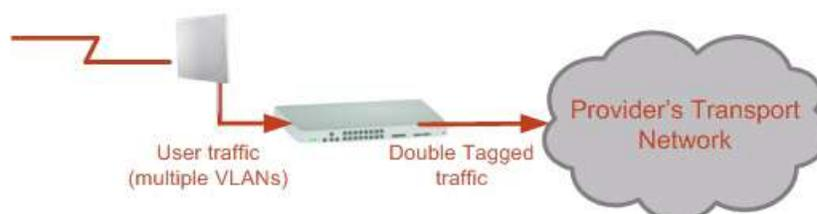
With this setting, ingress frames which are not tagged with the configured provider VLAN ID are blocked (filtered).
