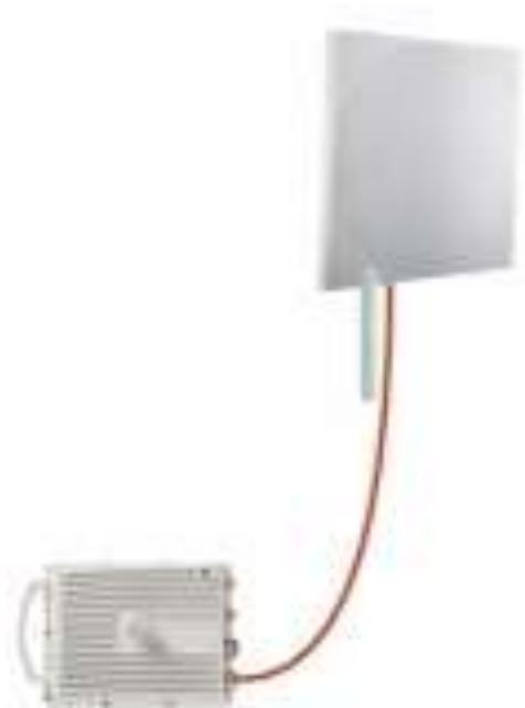
Figure B-5. Incorrectly Mounted ODU (No "Water Nose")
