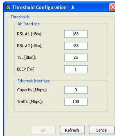
Figure 5-2. Threshold Configuration Dialog Box
