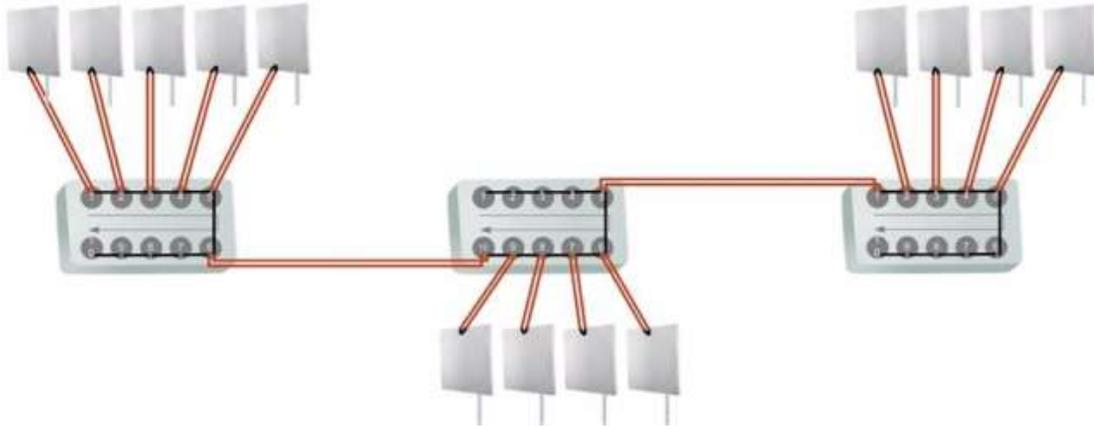
Figure G-8. Cascading Three HSS Units
