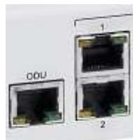
*Figure 2-8. LAN Ports on the Front Panel of the IDUE*
