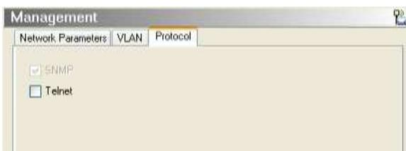
Figure 3-5. Enabling/Disabling Telnet Access
