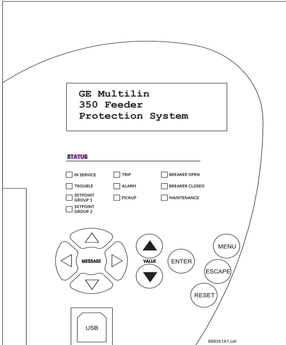
Figure 2: 350 Feeder Protection System Front Panel - Programmable LEDs
