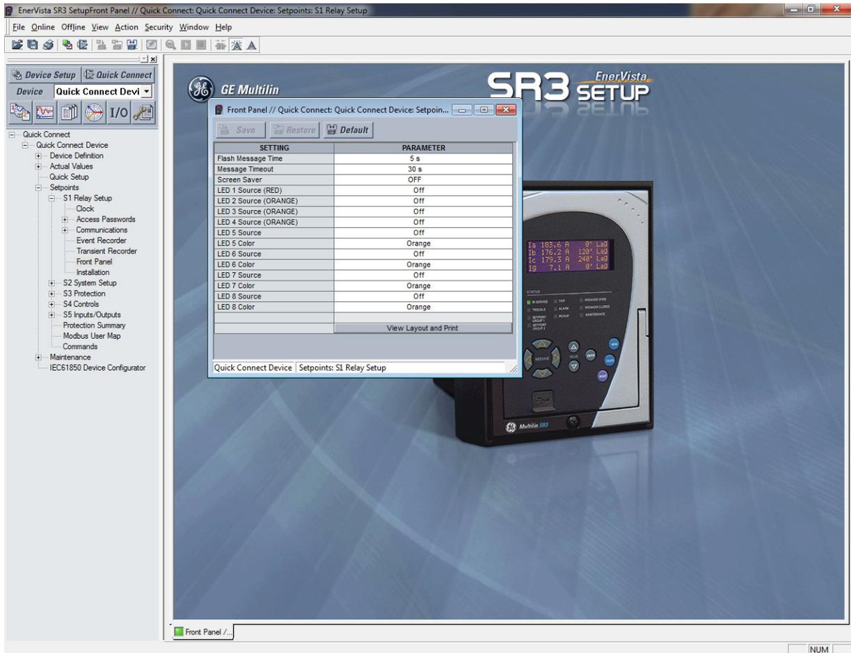
4. The Front Panel settings window opens with a corresponding status indicator on the lower left of the EnerVista SR3 Setup window.
