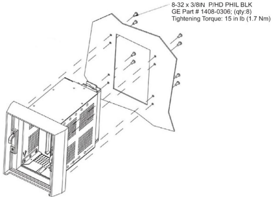
Figure 5: Standard Panel mounting - Non-drawout
