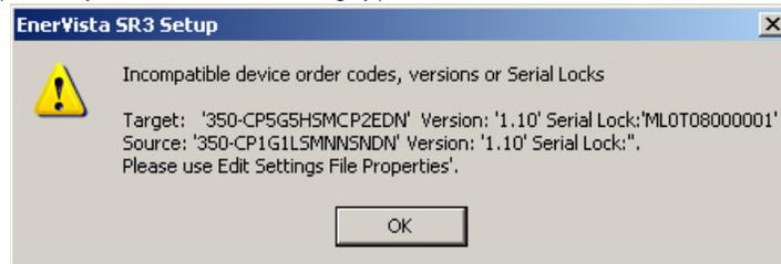
If there are no incompatibilities between the target device and the settings file, the data will be transferred to the relay. An indication of the percentage completed will be shown in the bottom of the main window.
