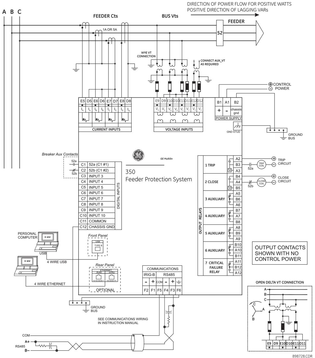
Figure 13: Typical wiring diagram - Non-drawout
