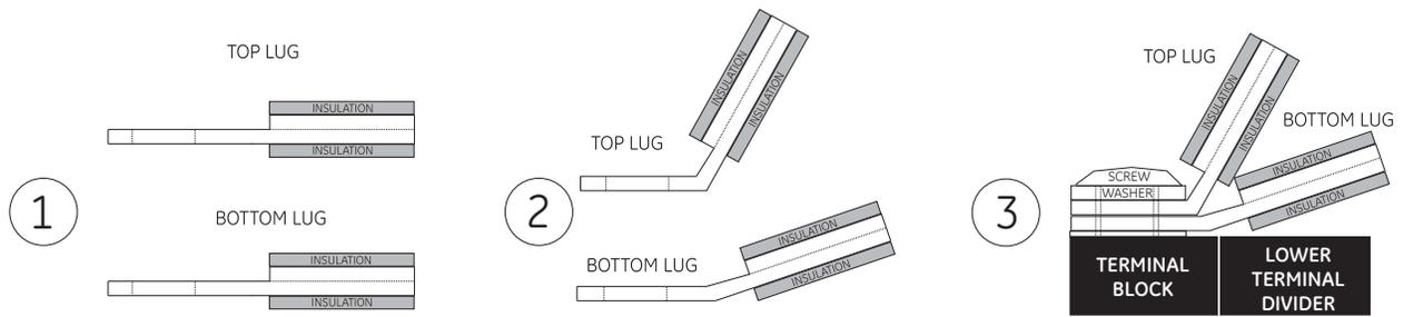
Figure 15: CORRECT INSTALLATION METHOD
