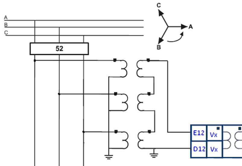
When "Voltage" polarization is selected, the direction is determined by comparing the angle between the operating current and the voltage, and the set MTA angle. In cases where the voltage drops below the setting of the minimum polarizing voltage, the neutral directional element is undefined (see following table).
