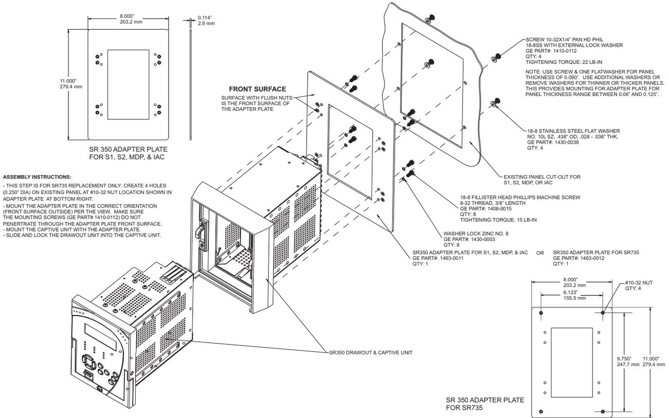
Figure 9: Non-drawout - Adapter plate mounting
