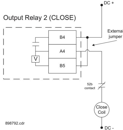
**Example 2:** Some applications require that the Close Coil be monitored continuously, regardless of the breaker position (open or closed). This can be achieved by connecting a suitable resistor (see the table) across breaker auxiliary contact 52b in the Close circuit. With such connections, the trickle current will be maintained by the resistor when the breaker is closed. For these applications the setting for "BYPASS BKR STATUS" should be set to ENABLED.
