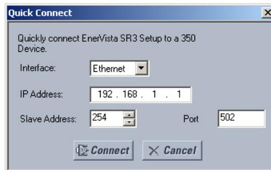
As indicated by the window, the "Quick Connect" feature can quickly connect the EnerVista SR3 Setup software to a 350 front port if the USB is selected in the interface drop-down list. Select "350 Relay" and press the **Connect** button. Ethernet can also be used as the interface for Quick Connect as shown above.
