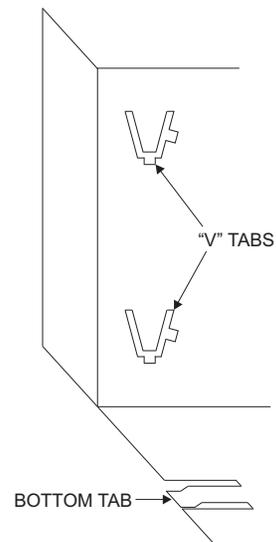
1. From the front of the panel, slide the empty case into the cutout until the bottom tab clicks into place (see above).
