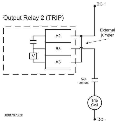
**Example 2:** Some applications require that the Trip coil be monitored continuously, regardless of the breaker position (open or closed). This can be achieved by connecting a suitable resistor (see the table) across breaker auxiliary contact 52a in the trip circuit. With such connections, the trickle current will be maintained by the resistor when the breaker is open. For these applications the setting for “BYPASS BKR STATUS” should be set to ENABLED.
