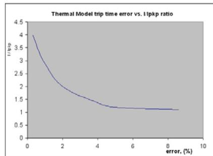
The graph shows the trip time error with respect to the ratio of cable load and thermal model pickup setting. With a smaller  $I/lpkp$  ratio, the time error tends to be higher, as accumulated through the logarithmic formula, the measurement error, and the time of measurement. For higher  $I/lpkp$  ratios, the time to trip is substantially more accurate. Each point on the graph represents a trip time error, with the  $I/lpkp$  ratio kept constant during the test.
