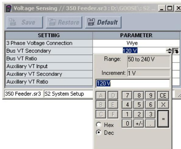
5. For setpoints requiring non-numerical pre-set values (e.g. **3-Phase voltage connection** below), clicking anywhere within the setpoint value box displays a drop-down selection menu arrow. Select the desired value from this list.
