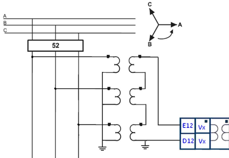
The fault is detected in the Forward direction when the direction of the operating current  $I_g$  is within  $\pm 90^\circ$  of the polarizing signal. Otherwise the direction is detected as Reverse.
