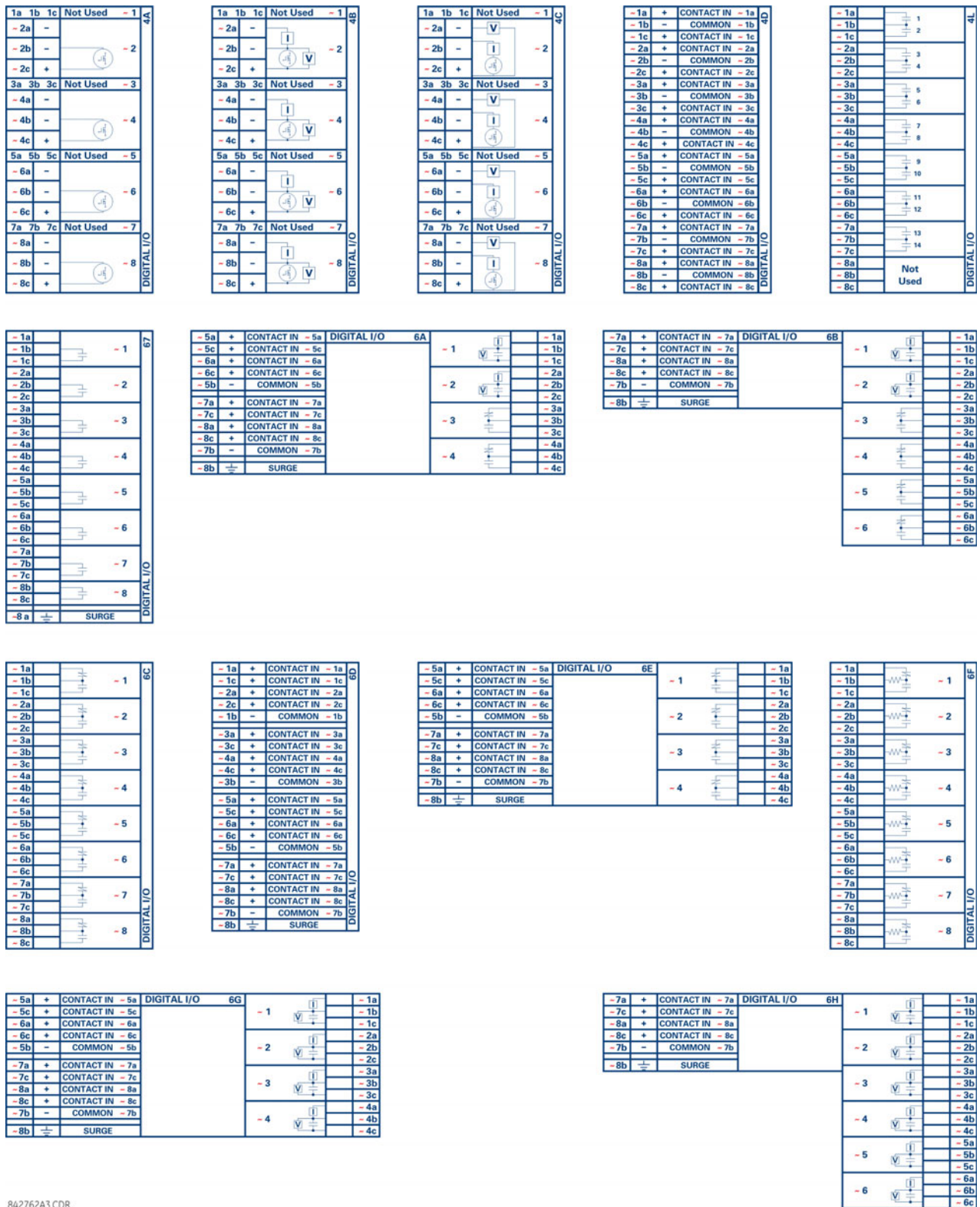
Figure 3-15: CONTACT INPUT AND OUTPUT MODULE WIRING (1 of 2)
