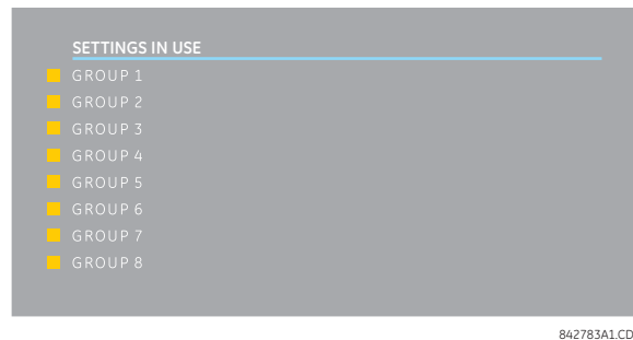
Figure 4-21: LED PANEL 2 (DEFAULT LABELS)
