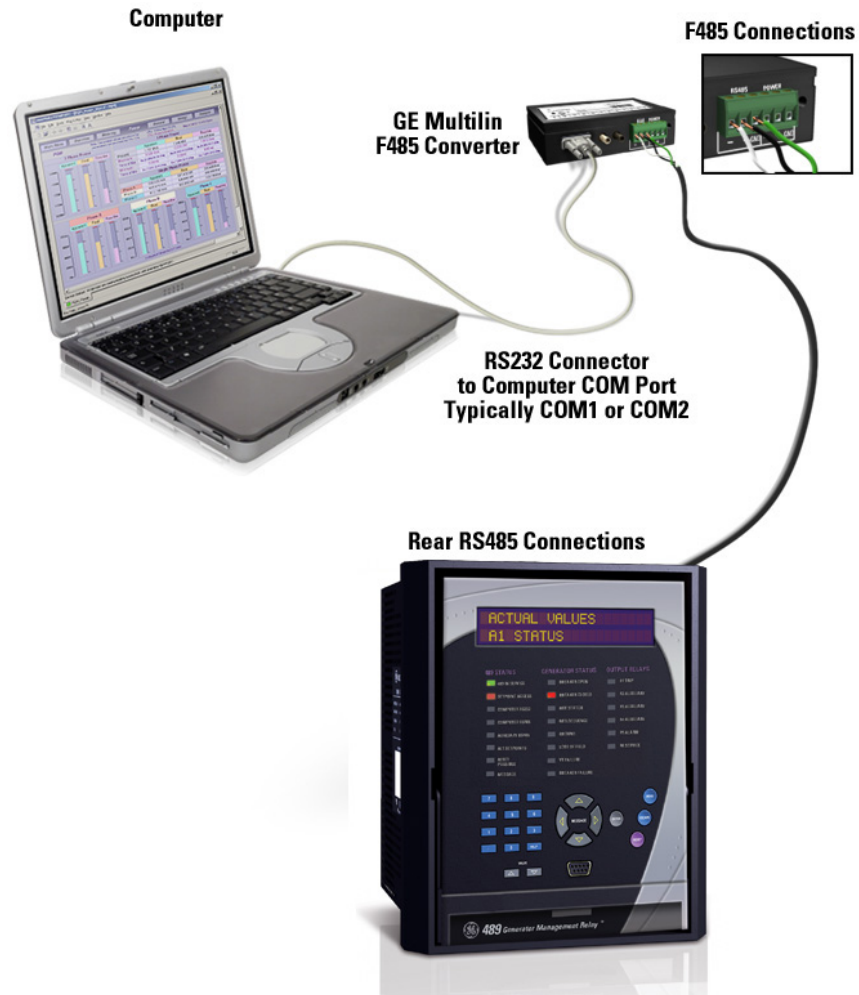
FIGURE 4-3: Communications using Rear RS485 Port
