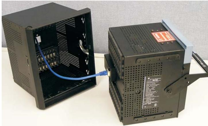
FIGURE 3–10: Ethernet Cable Connection
