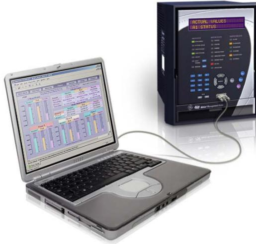
FIGURE 4-2: Communications using The Front RS232 Port
