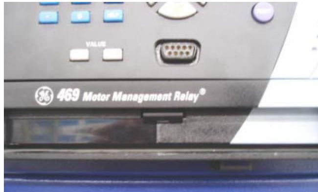
FIGURE 3-2: Seal on Drawout Unit
