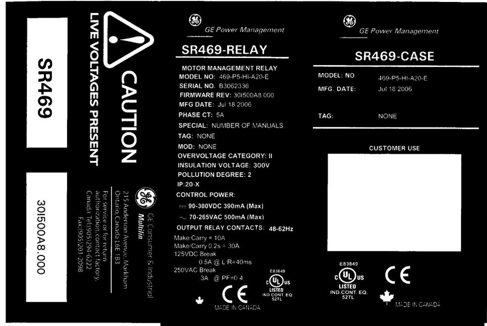
FIGURE 3–3: Case and Unit Identification Labels
