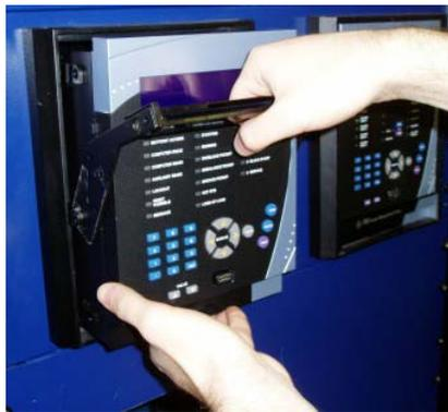
**FIGURE 3-9: Slide Unit out of Case**
